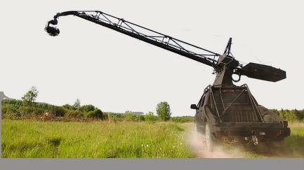
weighing more than 85kg. Light and agile Black Unicorn Crane allows shooting at a carrier speed of over 180 km/h and 90 km/h off-road. Remote control of the crane is carried cut from the cabin of the vehicle. Black Unicorn Crane is not difficult to uninstall from the roof of the car and to install on other vehicles of various types, for example, on a boat or a train.
