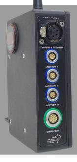
Remote lens control system has mechanical limits of focus and iris channels. Automatic calibration of high precision lens is achieved by pressing a button. A built-in battery allows to operate for 24 hours without an interval. The device is to be used with 1 – 3 Heden motors and operates Canon or Fujinon digital lens. Control operating distance via radiochannel reaches 1km in the direct sightline.
